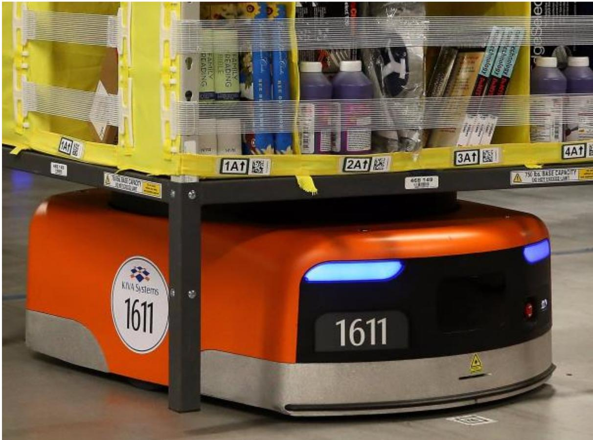
Amazon's Kiva co-bots don't replace human pickers and packers but, by moving the goods around the warehouse more efficiently, they reduce human walking time. Each Kiva robot weighs 320lb (145kg) and can carry the weight of a small car. These co-bots take their instructions by scanning QR codes
