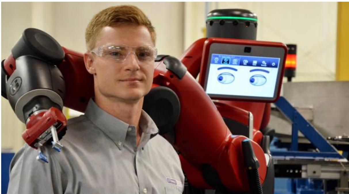
Stationery co-bots often work on packaging and electronics assembly lines, moving items across conveyor belts, inserting products into boxes, inserting components into a circuit board, or carrying out quality control checks.
